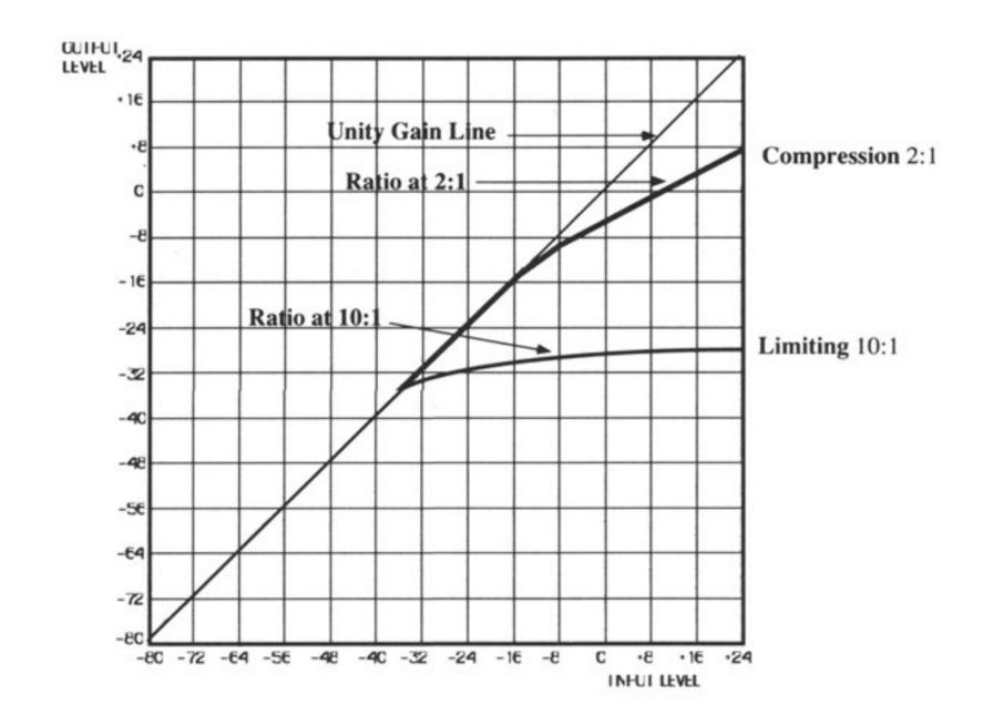
Two plots are shown, representing the gain curves of two different setups using the UREI LA-10 or LA-12. The bold lines represent a deviation from unity gain caused by compression. At low signal levels, the gain curves are identical. When the input signal is above -36 dBu, the curves separate, indicating different threshold and ratio settings.
